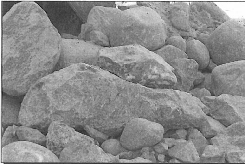
Photo 3 Mixture of round rock and blasted granite ready for placement at bridge site
