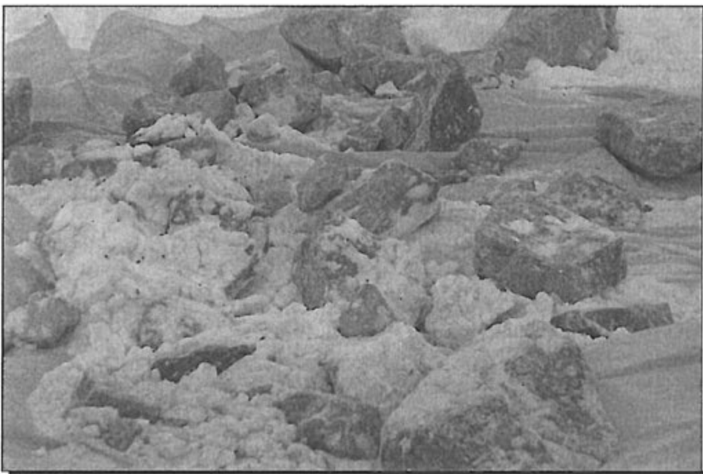
Photo 2 Blasted granite spread out and sorted according to size
