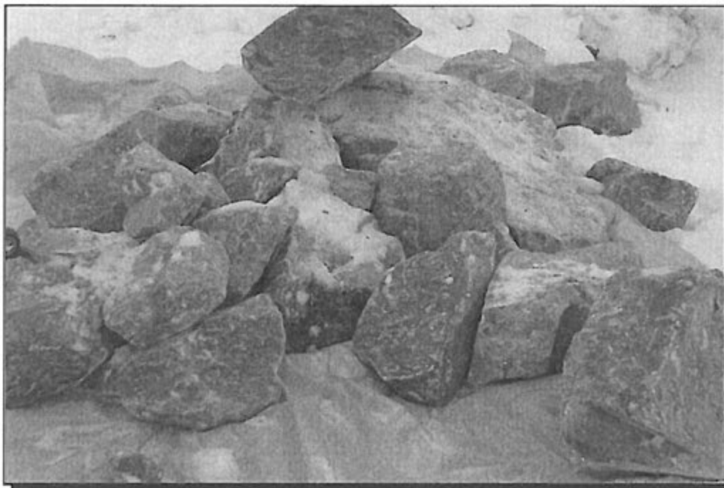
Photo 1 Blasted granite placed on tarp for gradation test
